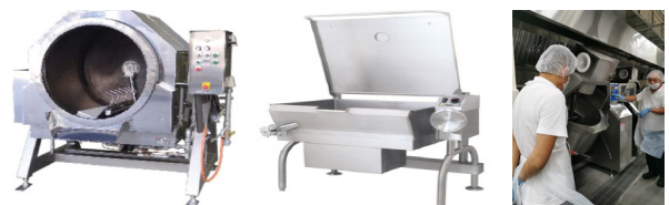
Revolving cooker and tilting braising pan cuts down on labour-intensive work (only involves 2 staff).
