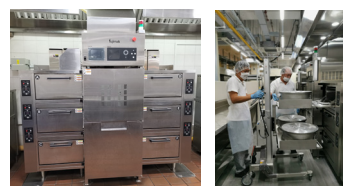
Automated Rice-Pro machine which can handle the washing of rice to cooking and segregation of rice (only involve 1 staff).
